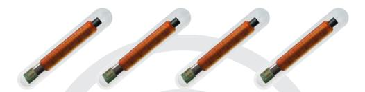
Microchips come in various shapes and sizes, however, Pet-ID Microchips advocate the use of 12mm chips for companion animal identification. Manufactured to ISO 11784/11785 and encased in bio-compatible glass, our microchips are coated with Parylene-C, a medical grade coating, which forms an irregular surface allowing tissue fibres to bond and grow around the chip, preventing the possibility of migration.
